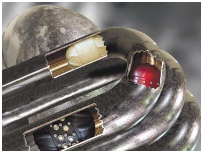
FIG. 7 Piggging options for quick and easy mechanical decoking. (Photo courtesy of Eveready Energy Services)
