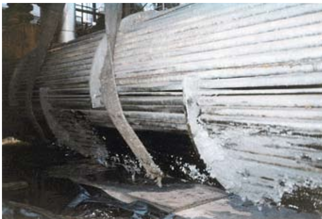
FIG. 11 Conventional exchanger in bitumen service—fouled after nine months.
